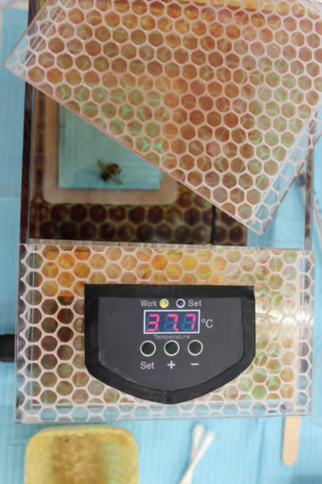
BICU / Bee, I See You / Bee Intensive Care Unit: Prototype #2, 2018 Laser-etched plexiglass, beeswax foundation sheets, incubator components (heating element, temperature controller, sensor, and fan) 5 x 7 x 3 in
